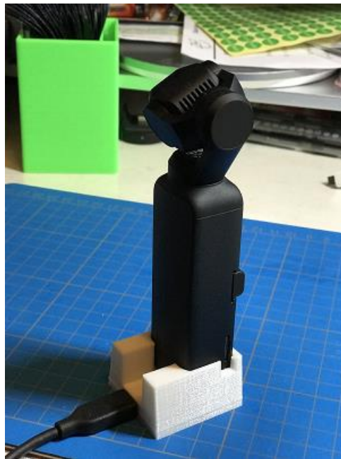
Figure 3: Example of using the USB3.1-CMV-CF-V1A to build a USB3.1 Type C charger dock with 3D printed case.
